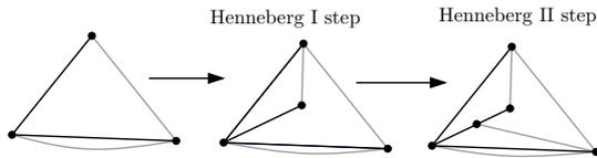
Figure 6: Constructing a decomposition into two spanning trees via Henneberg steps.
